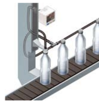
Air-leak test for PET bottles
